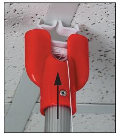
Lift Installation Pole up to ceiling grid. Push up until clip snaps closed.
