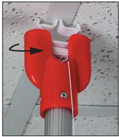
To release Eagle™ Ceiling Clip, rotate pole until clips springs open. NOTE: Do not push up on clip when rotating.
